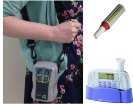
**Figure 1: The Personal Air Monitor (PAM) being carried on the left, peak flow meter (top-right) and spirometer instruments (bottom-right) (without case).**
